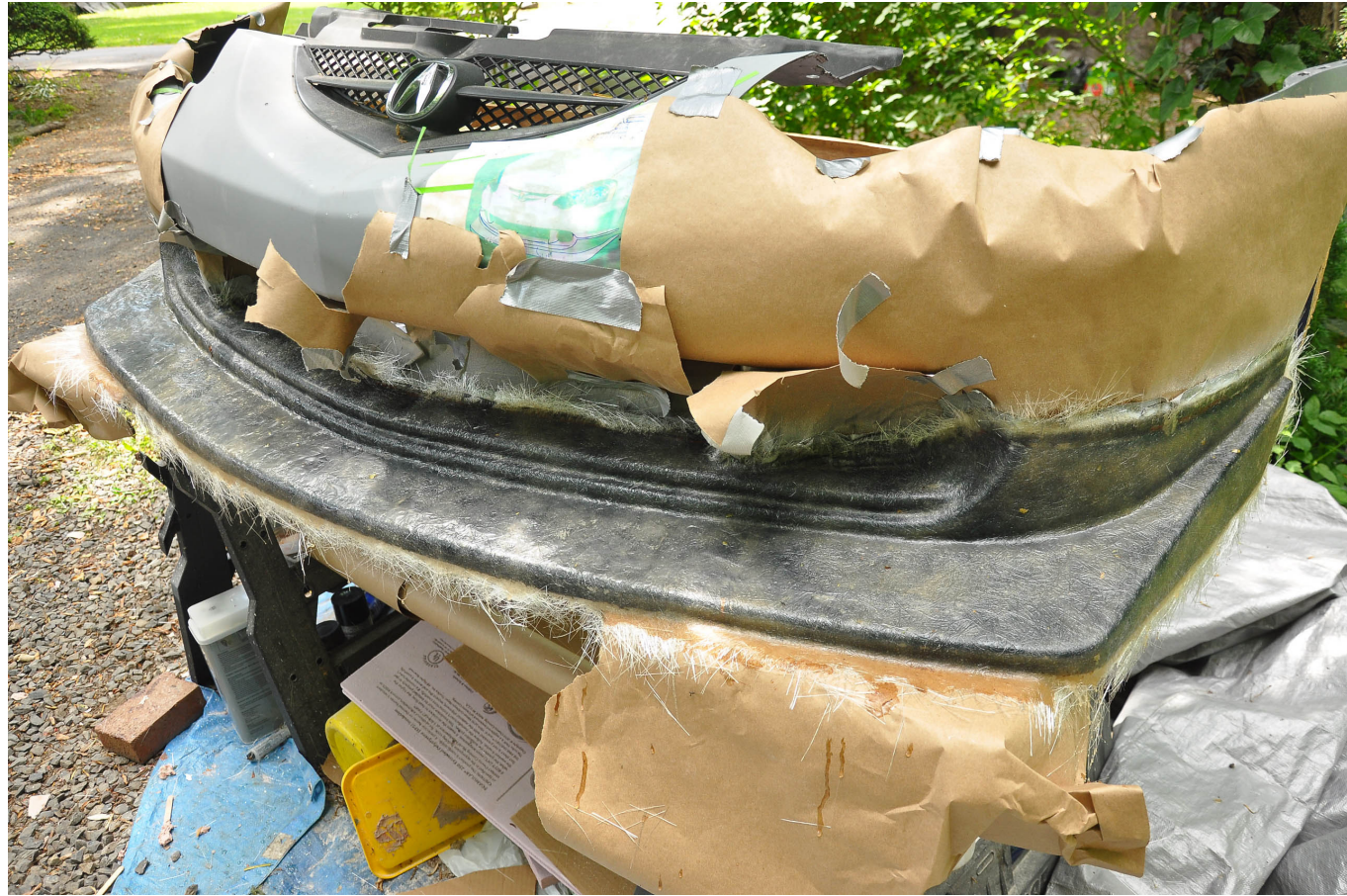
A fiberglass outer shell is added to the prototype, which also joins the fiberglass base and the outer shell into one piece.
