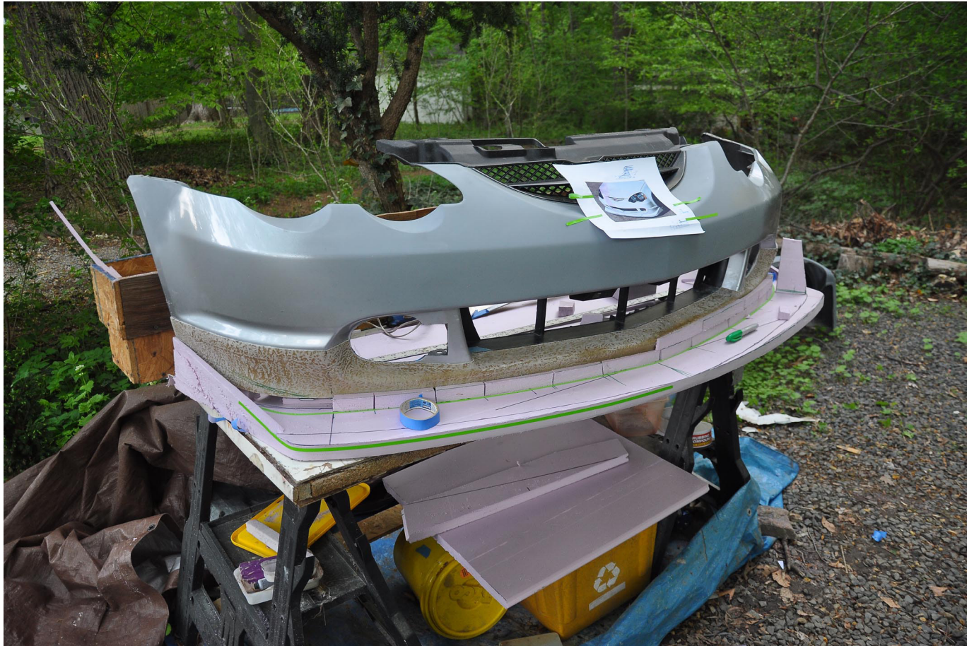
Fiberglass prototype base has been scuffed for adhesion and foam has been attached to create the lower portion of the design. Tape is used to mark out the detail lines.
