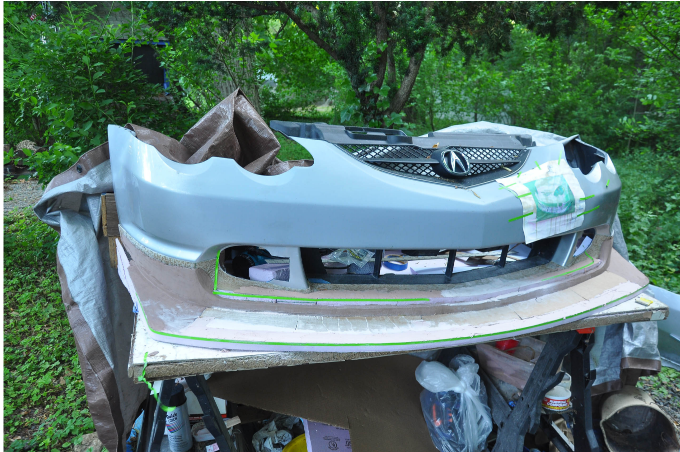
Chavant clay is used to block in surface transitions and detail lines. This prototype will be finished with a fiberglass shell, so the clay isn't used for the finishing surface.
