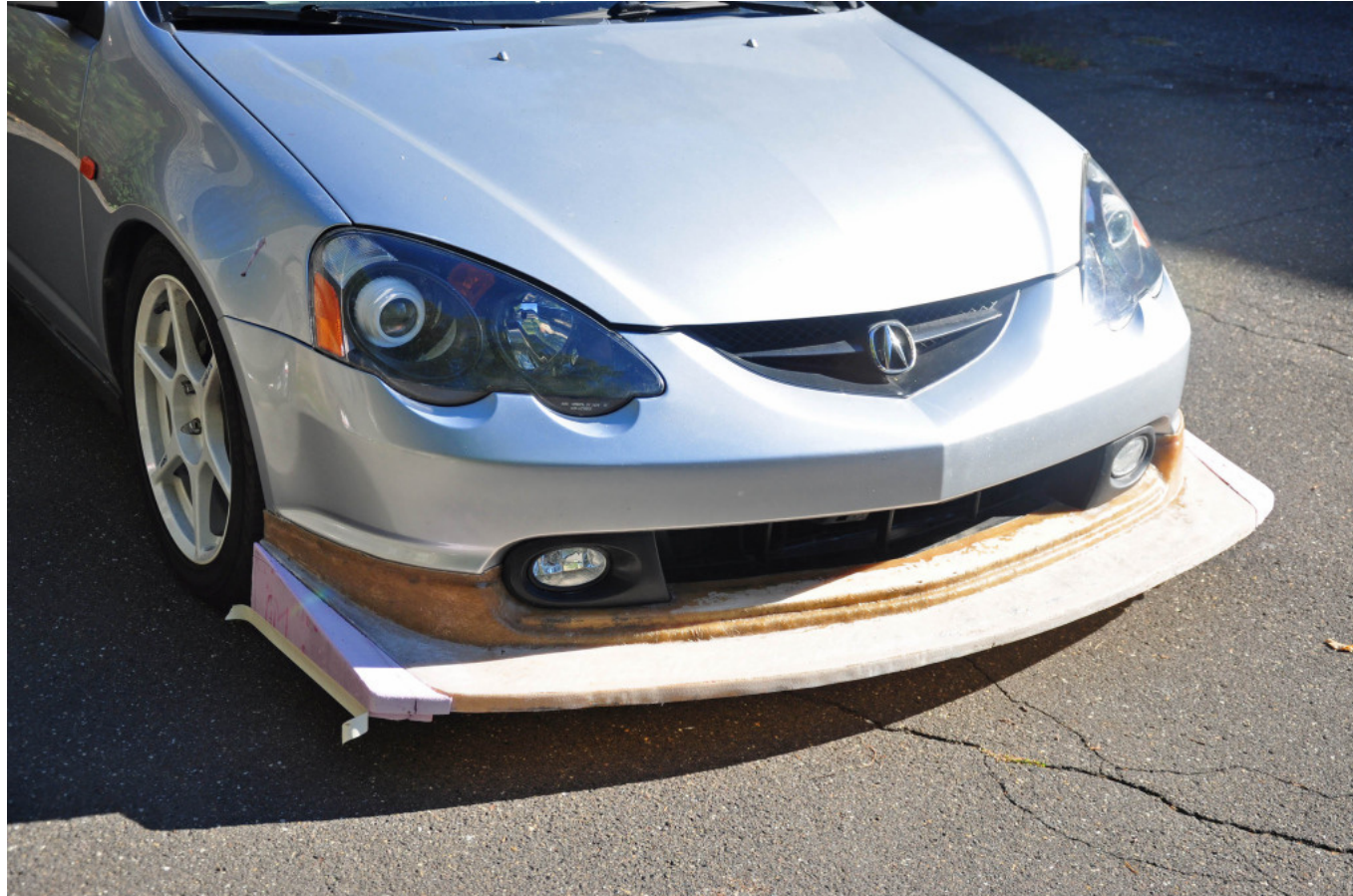
This photo shows the lip splitter mounted to the car, with foam extension pieces added to both sides as an after thought. These pieces add more surface area and create a 90° degree angle from the wheel well to the side surface of the lip.
