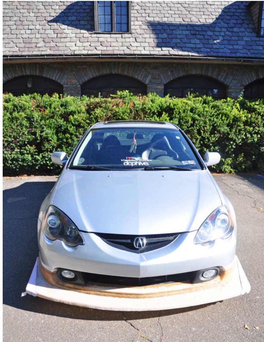
Front view of the lip splitter showing the large amount of surface area it has and the overall width of the piece. The optional factory fog lights fit perfect with no interruption from the lip splitters mounting.
