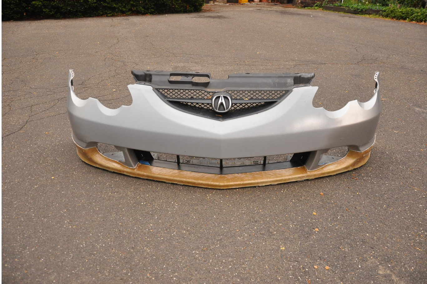
Fiberglass prototype base made to fit snug to the bumper to ensure proper fitment. This is used for just the prototype, the finished parts will not have this base.
