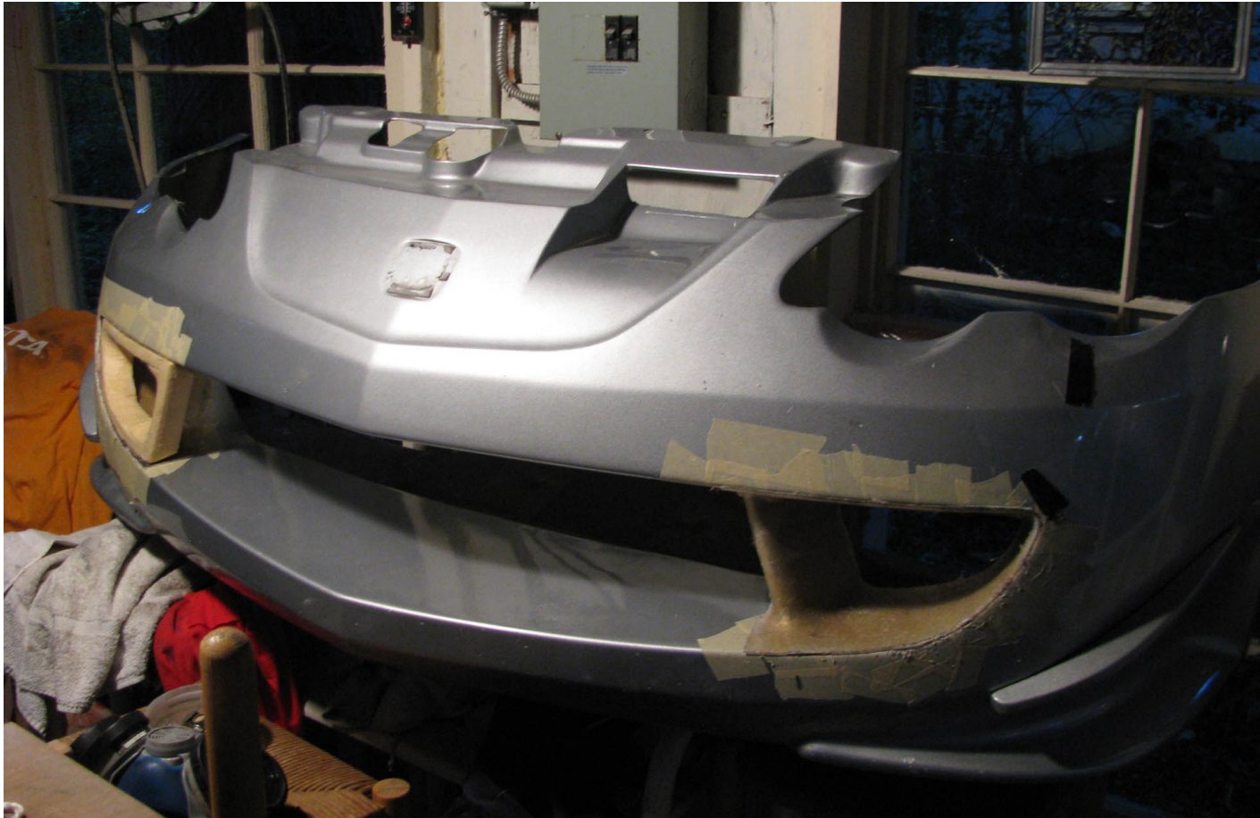
Early prototype phase: Both airdam ducts have been given a fiberglass base, and the start of the exterior housing for the foglights has begun.
