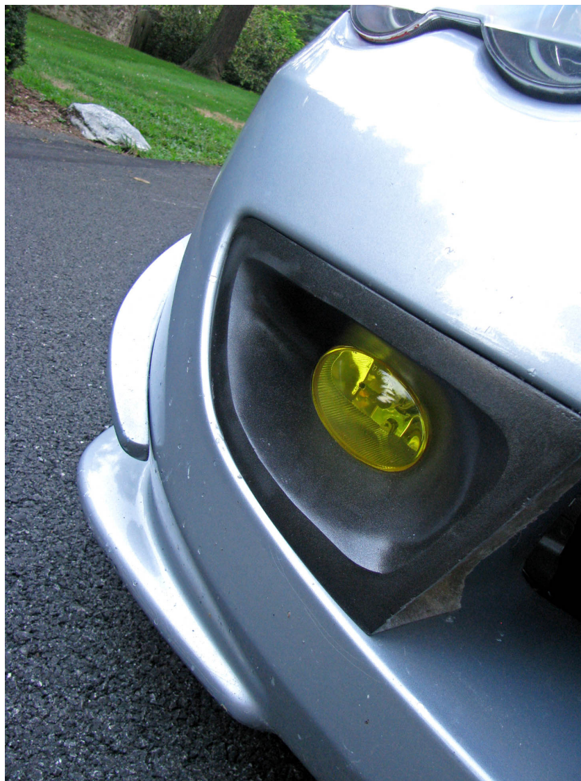
Another closeup shot showing the refined housing fitted with the fog light into the side airdam of the bumper. The side return still needs to be added to make the housing complete.
