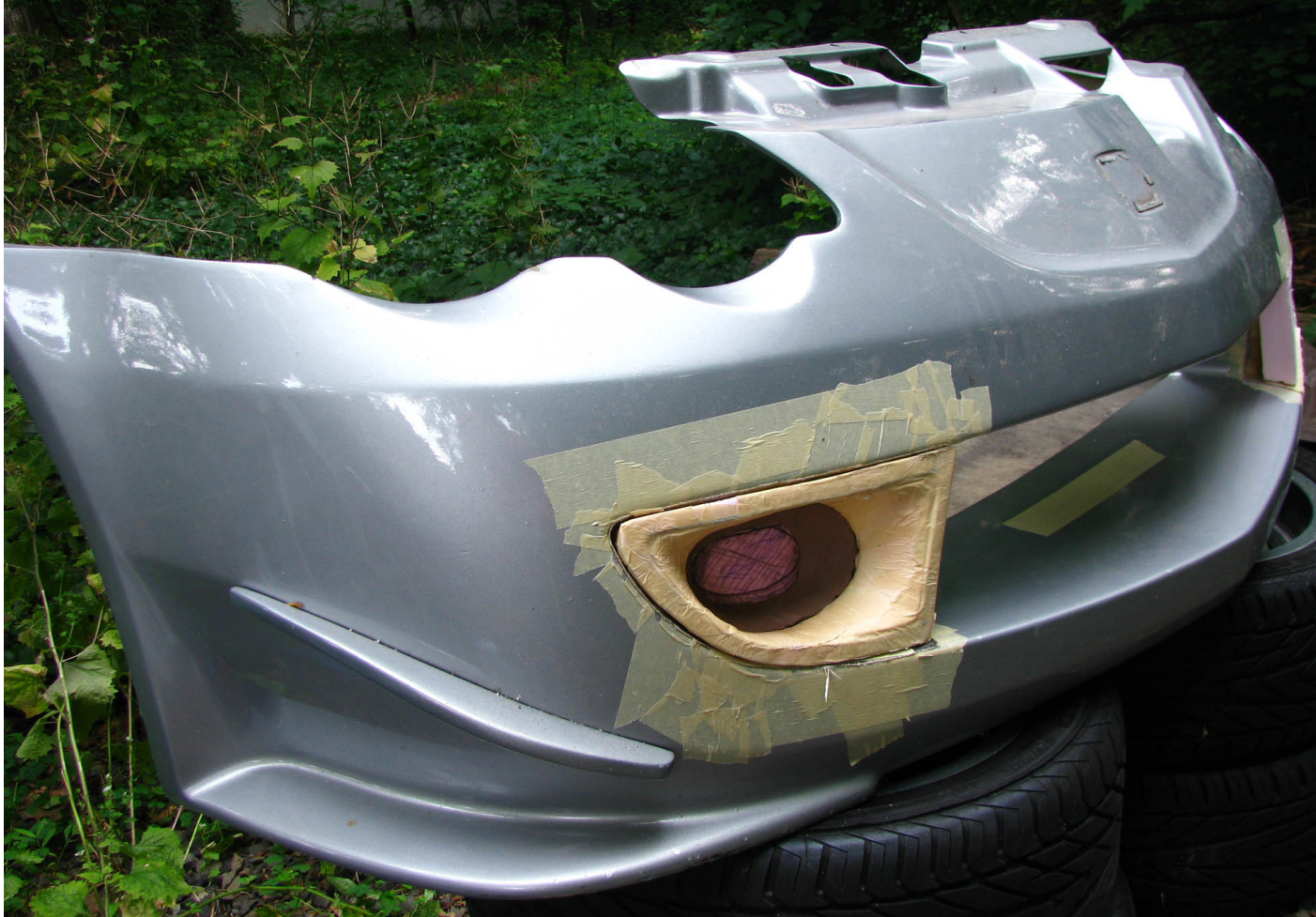
A template has been made of the outside shape of the fog light, and transferred onto a backing board. Clay was then used to transition the form from the outer housing to the light itself.
